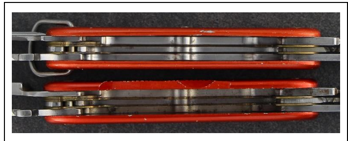
Photo top left: Different boards/interlayers from brass-brass to brass-nickel silver to nickel silver-nickel silver. Photo top right: old variant below with external awl; Newer variant at the top with an internal awl
