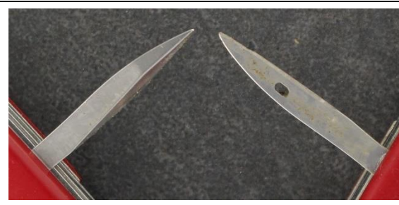
The awls of the two pocket knives are completely different. The awl from Henckels on the left is very simple without any advanced functions.
