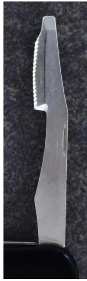
Coarsely serrated cutting edge, smooth surface
