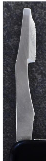
Coarsely serrated cutting edge, smooth surface
